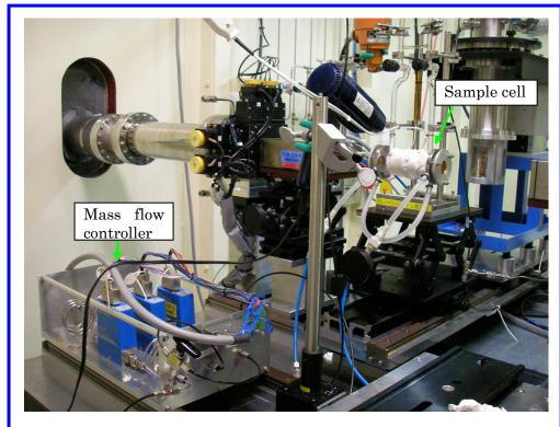
Fig. 5 Setup of in-situ XAFS equipments
