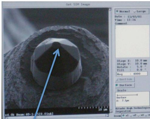
Culet diameter : 3 μm
