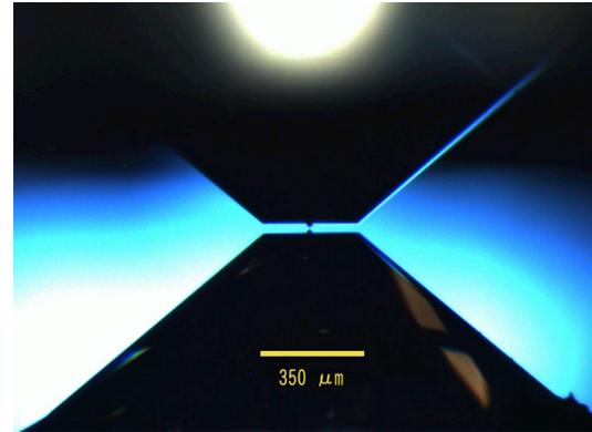
Micro anvils placed on top of normal anvils (350 μm culet)
