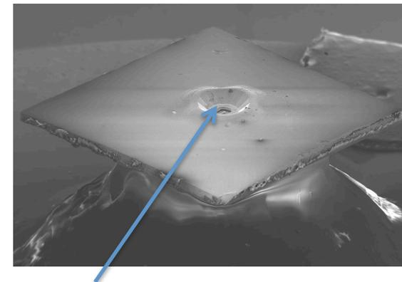
Gasket hole was filled with liquid
