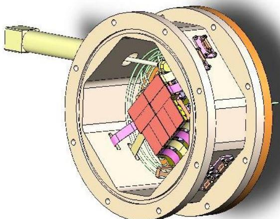
Octal Sensor Detector ( $100 \times 100 \text{ mm}$ )
