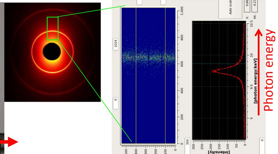
Wavelengths ( $\lambda$ ) are calculated from positions of Debye-Scherrer rings on MPCCD.
